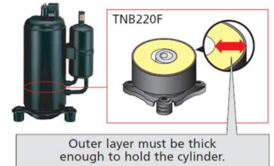
Compressor Using Conventional Method (Arc Spot-Welded Method)
