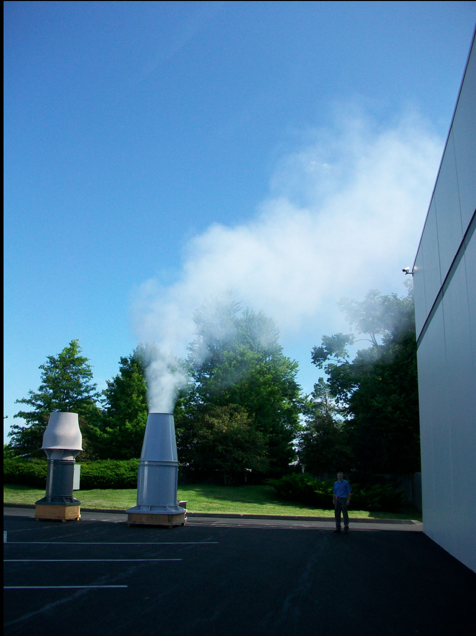
Fan with tapered discharge
